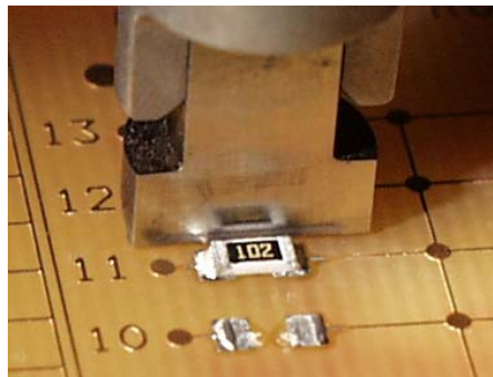
Figure 9. Shear test jig and push-off tool before a shear test
