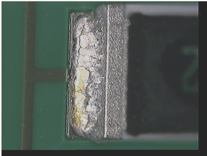
Figure 1. A 2512-type chip resistor showing cracking in the solder joint.
