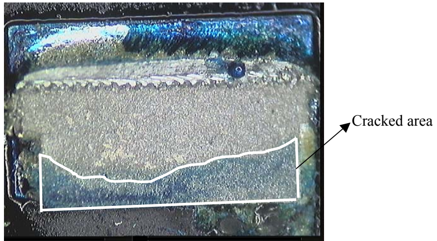
Figure 6. Crack in a SnAgCu solder joint after thermal cycling.
